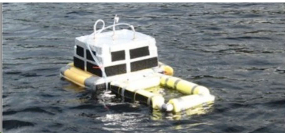
Floating chambers used by Peters Award recipient Dominic Vachon to measure CO 2 flux from lakes.
